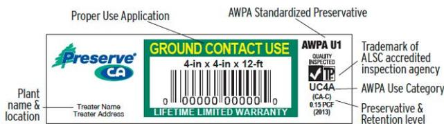
Treated lumber is either made for ground contact applications or above ground uses. Ground contact applications include posts and pilings buried in the earth, and also near-ground projects such as low-rise decks that are six inches or less from the ground. These applications require more protection against fungal decay and termite attack than above ground applications, so retention rates are higher on ground contact lumber.
