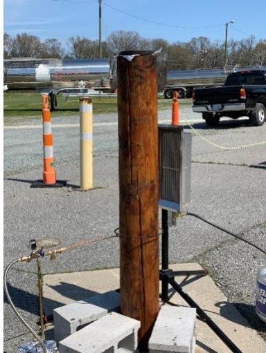
Fig. 1 Small-scale fire test apparatus for utility pole
