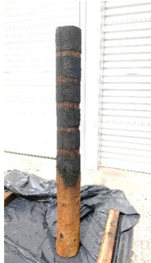
Fig. 3 Five marked locations for cha depth measurement
