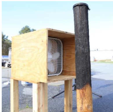
Fig. 2 wind exposure for post-burn utility pole
